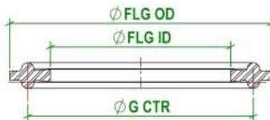
GASKET PROFILE FOR SIZES WITH A 34.0mm FLG OD & ABOVE (UNLIPPED VERSION)
